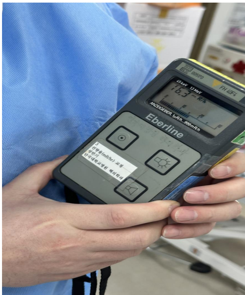
Supplementary Fig. 1. Radiation dose rate at the trunk-mounted personal dosimeter position, showing approximately 0.16 mSv/h.
